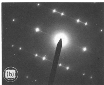
Figure 3 (a) Dark-field image of whisker segment showing high and low defect density regions of varying length in twin relations; (b) \langle 110 \rangle SADP from region labelled in (a).
